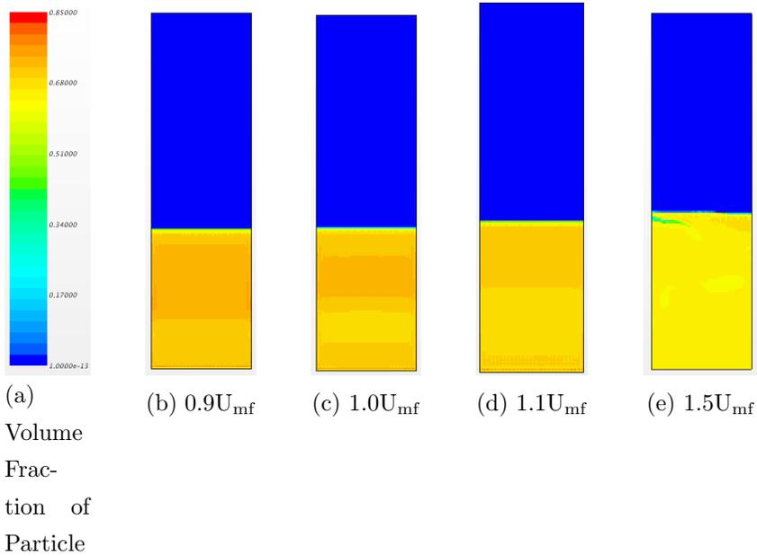
Figure 1: Solid Volume Fraction snapshots at different fluidization velocities ( $C_1=0.8$  and  $C_2 = 2.65$ )
