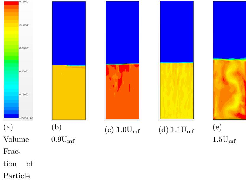
Figure 3: Solid Volume Fraction snapshots at different fluidization velocities (modified  $C_1=7.23$  and  $C_2 = 0.38$ )
