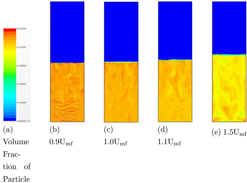
Figure 2: Solid Volume Fraction snapshots at different fluidization velocities (modified  $C_1=9$  and  $C_2 = 0.28$ )
