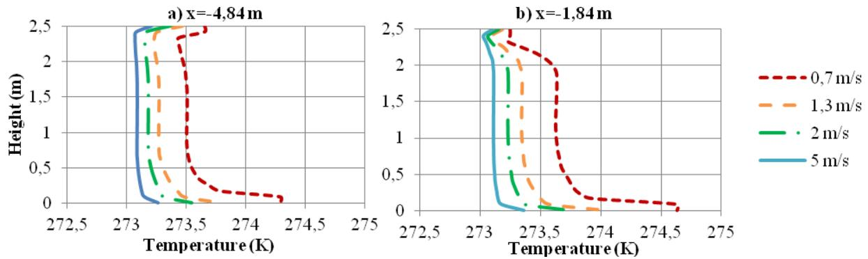
Figure 8: Influence of blowing velocity on vertical temperature profile.
