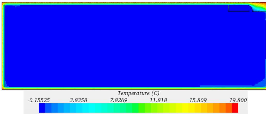
Figure 10: Temperature field of the compartment, including the insulated walls.
