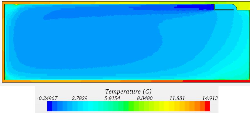
Figure 11: Temperature field of the compartment, including the insulated walls.
