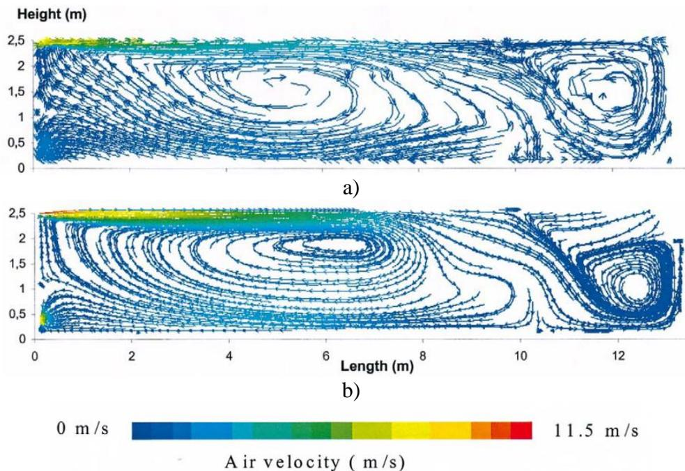
Figure 1: Velocity field in the refrigerated truck (Moureh *et al.* 2002)
