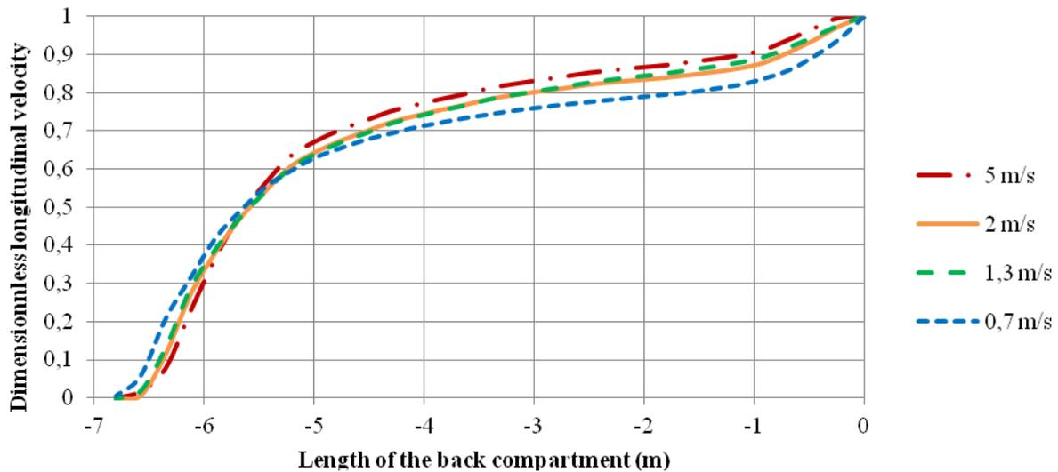
Figure 7: Longitudinal velocity on the jet axis along the truck enclosure ( $y=2.4$  m).
