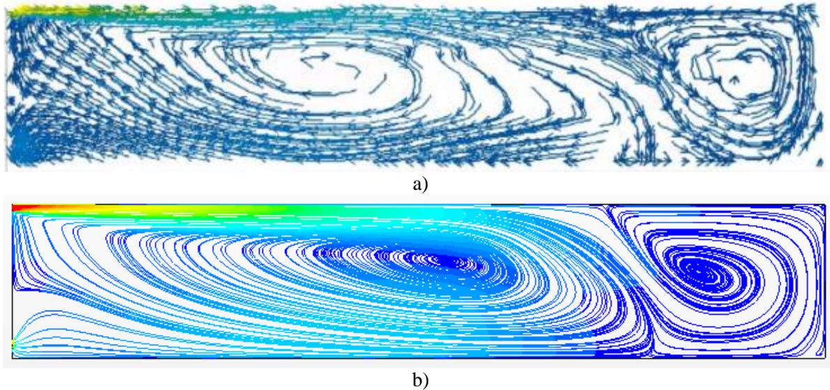
Figure 4: Velocity stream lines in the refrigerated truck,
