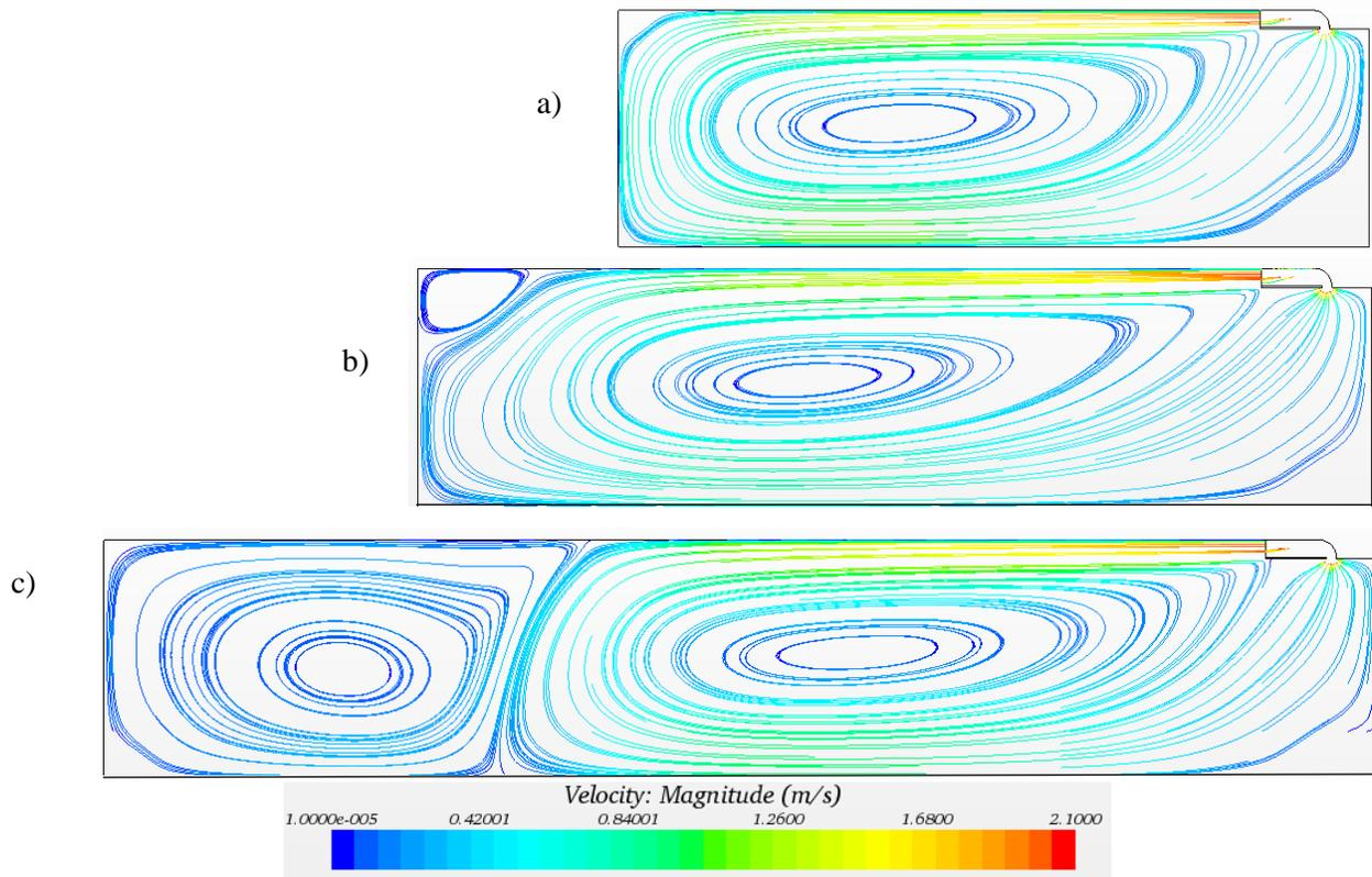
Figure 9: Velocity streamlines for three back compartment lengths: a) 8 m, b) 10 m, c) 13.3 m.
