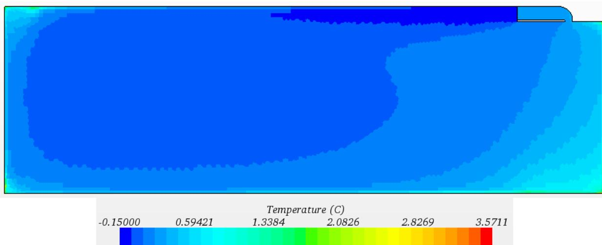
Figure 5: Temperature field of the compartment (heat flux: 10 W/m<sup>2</sup>)
