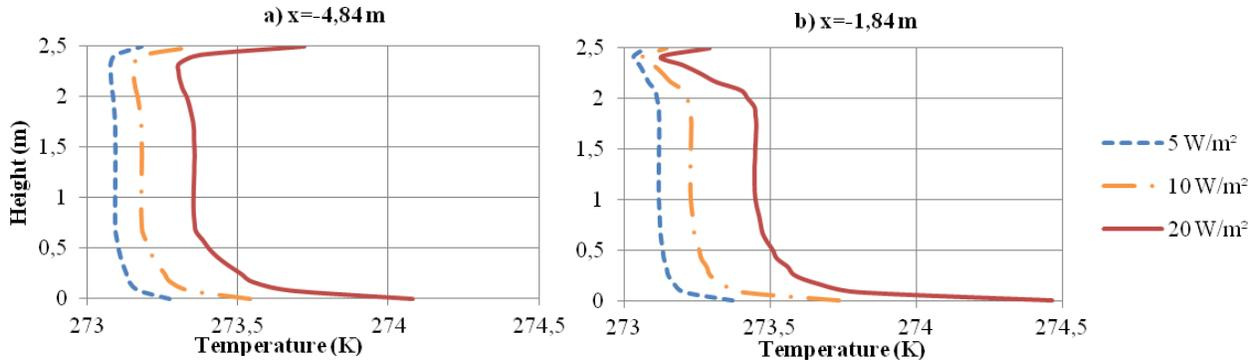
Figure 6: Influence of heat flux on vertical temperature profile.
