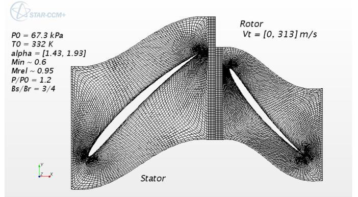
FIGURE 1. COMPUTATIONAL MESH FOR TWO-DIMENSIONAL COMPRESSOR STAGE.
