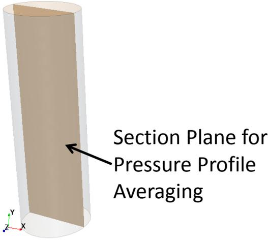
Figure 2: Section Plane for Pressure Profile Averaging
