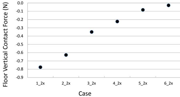
Figure 10: Bottom Surface Contact Force for Scaled Model
