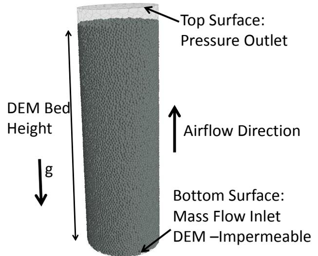
Figure 1: Computational Domain filled with Full Scale Particles
