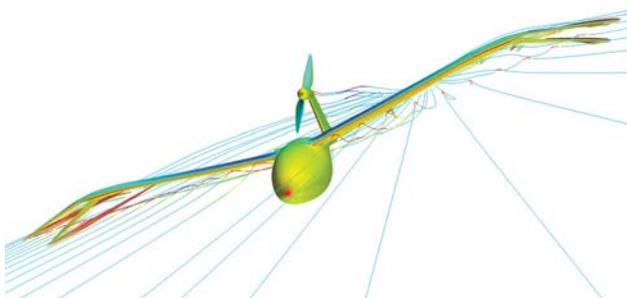
**FIGURE 5:** CFD analysis of the Lotus in cruise configuration
