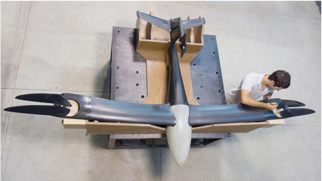
**FIGURE 3:** The Lotus during assembly, in cruise configuration
