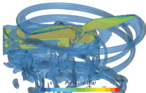
**FIGURE 6:** CFD analysis of the Lotus wingtip propeller at takeoff
