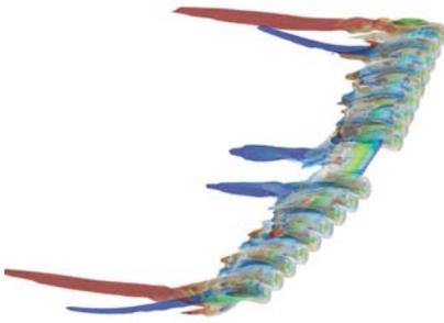
**FIGURE 7:** CFD simulation of the LEAPTech wing at takeoff; the propellers are modeled with actuator disks.
