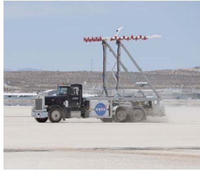
**FIGURE 8:** The LEAPTech experimental test apparatus at NASA Armstrong (NASA photo)
