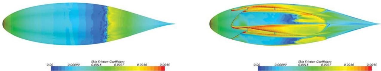
FIGURE 2: CFD analysis of the S2 nacelles, showing a clean nacelle (left) and a nacelle with folded blades and spinner gaps (right)
