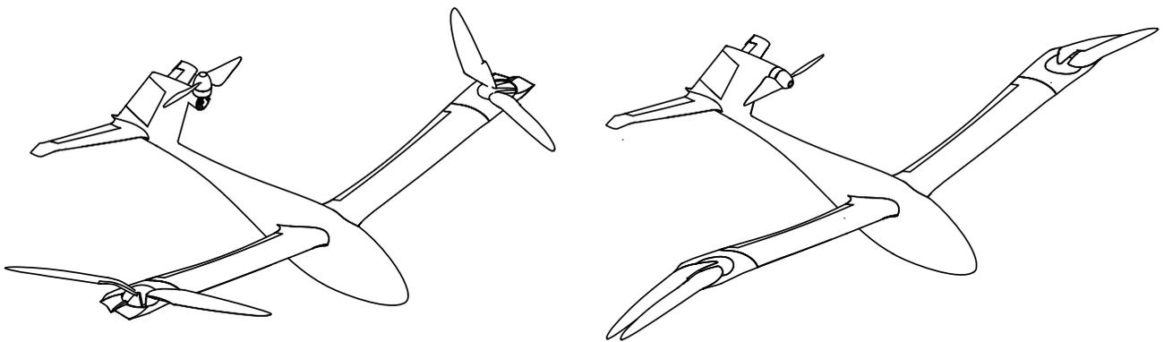
**FIGURE 4:** The Lotus in takeoff (left) and cruise configurations (right)
