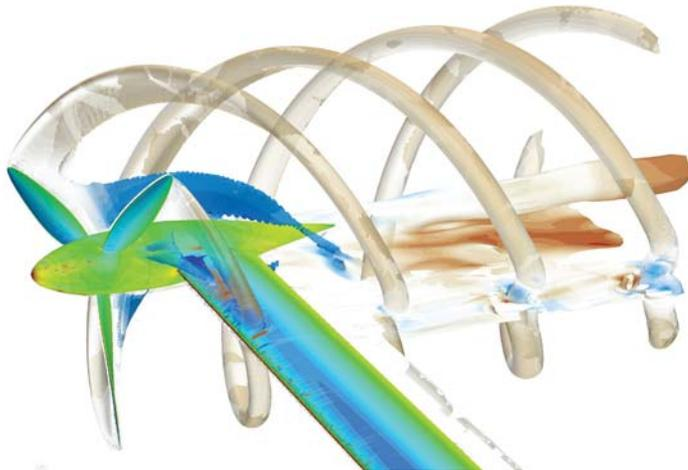
**FIGURE 9:** CFD simulation of a wingtip propeller
